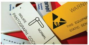
All types of computerised and manual machine engraving is currently available utilising a host of materials including aluminium, brass, stainless steel, perspex, engraving plastic (traffolite) and most other metals and plastics.
